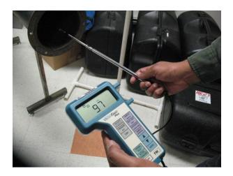
This photo shows a meter with a telescoping probe cable of displaying real-time data and/or logging data including air velocity, temperature, and humidity. This type of meter is often used when assessing ventilation systems.
